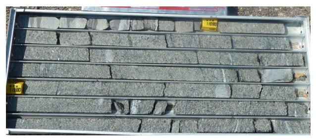
Figure 19. Magnetite garnet schist (MGS)
