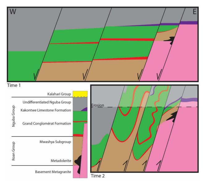
Figure 21. Schematic cross sections illustrating a structural model for the Xaudum area. During Time 1 synsedimentary normal faulting resulted in thickness changes within the Katangan Supergroup sequence and stratigraphic pinch outs over basement highs. During Time 2 regional compression resulted in reactivation of the faults to form reverse structures with local zones of intense folding adjacent to the original basement highs.
