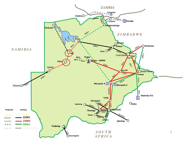
Figure 29. The Botswana national transmission grid expansion plan that is currently occurring, note the 132-kV line that is currently being built to Shakawe. After Thema, 2013
