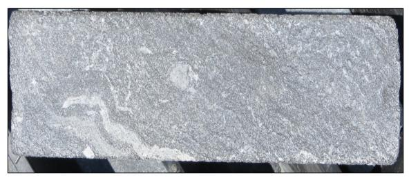
Figure 33. Magnetic Diamictite schist (DIM).
