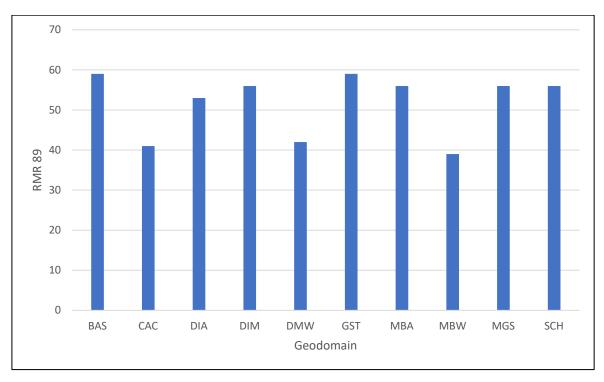
Figure 41. The graph representation of the Bieniawski RMR89 classification for the different Geodomains.
