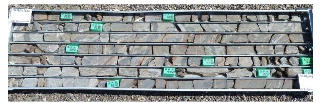
Figure 17. Weathered Banded magnetite
