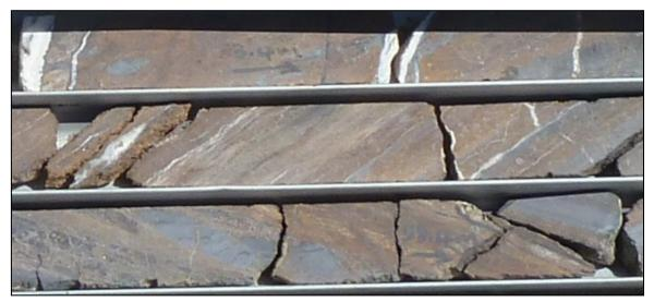
Figure 32. Weathered banded magnetite (MBW).
