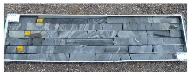
Figure 16. Banded magnetite - Geodomain
