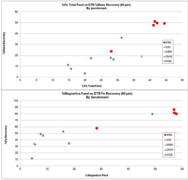
Figure 27. % Upper: Fe Head Feed (Total Feed) vs. the DTR % Mass Recovery, by Geodomain. Lower: % magnetics vs. % Fe Recovery, by geodomain. After Baker, 2014.
