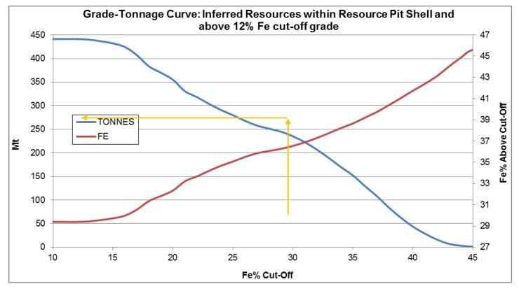
*Figure 9*. Shows the Grade Tonnage Curve for all Inferred material within (above) the Block 1 pit shell and above 12% Fe cut-off grade. Also show is the projected tonnage above a 30% Fe grade within Block 1 pit shells. After Baker, 2014.
