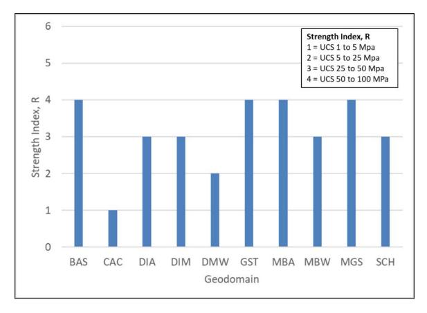
Figure 40. Intact rock strength of the different Geodomains.
