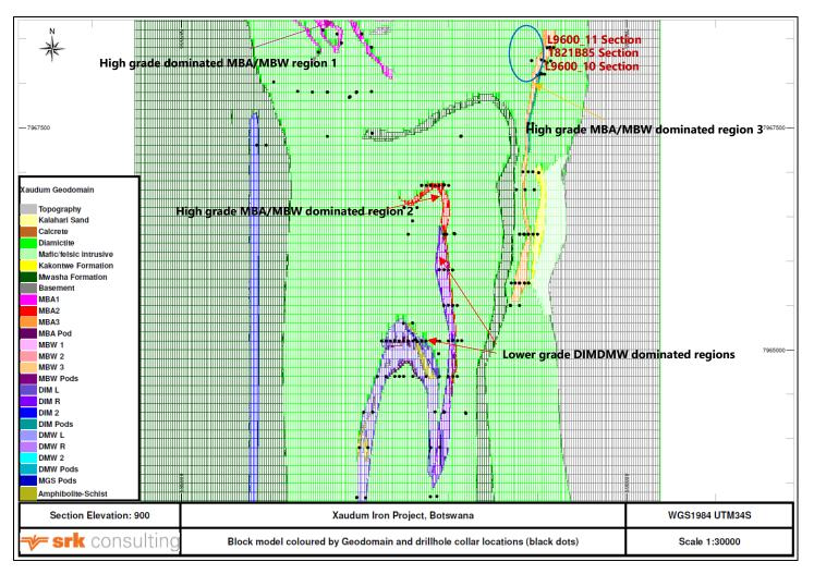
Figure 8. Highlighting the area (smaller blue oval and drill section labels) within Block 2 that Baker, 2014 suggested could be re-classified as Indicated without the need for extra drilling if one hole from each section was re-assayed using XRF analysis adding blind QA/QC samples. Taken from Baker, 2014, showing the drill collars and the 900 m RL block model colored by geodomain.
