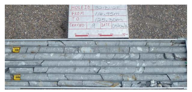
Figure 18. Magnetite diamictite schist (DIM)
