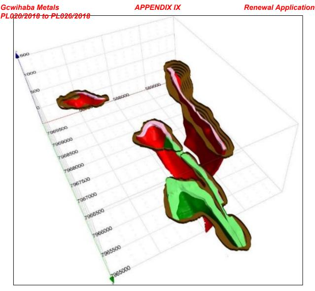
Figure 3. Diagram showing the main modelled XIF geodomains MBA (red), MBW (pink), DIM (green), and DMW (light green), and their respective grade within optimized pit shells.
