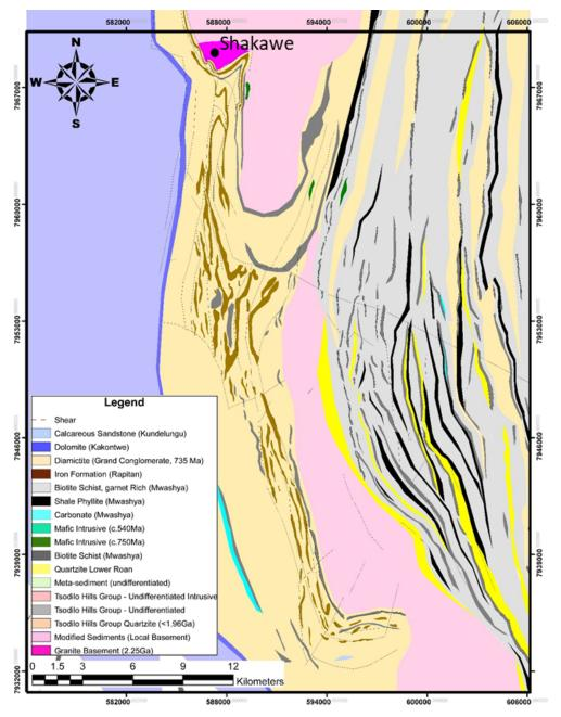
Figure 13. Local geology map showing main stratigraphic units and faults
