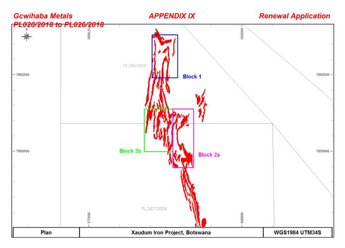
Figure 2. Showing the outline of the Xaudum Iron Formation mineralization body defined from ground magnetic geophysics. Shown also for reference are the Block 1 areas that has defined resources and the Block 2 area that will be the next area to be drilled for resource definition.
